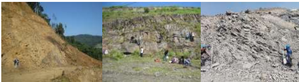
Figure 9. Thinly laminated, shale and mudstone with sandstone at the downstream
